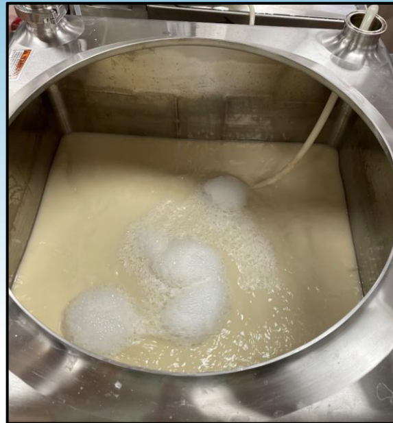
Batching of almond PBMA in Breddo Likwifier
